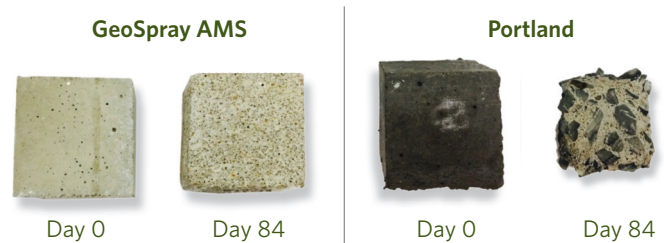
Figure 3. Portland Cement loses 50% of its mass when exposed to 7% Sulfuric acid, GeoSpray AMS is an order of magnitude better in performance
